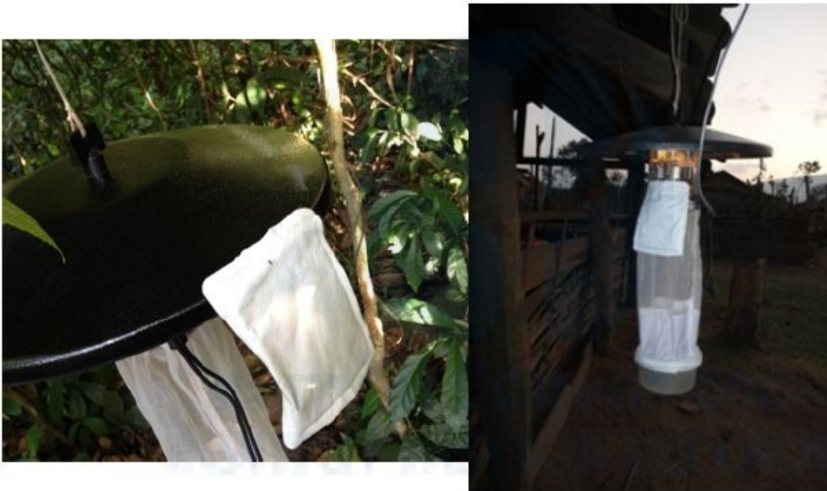
Figure 2: CDC light trap with heat pad.
