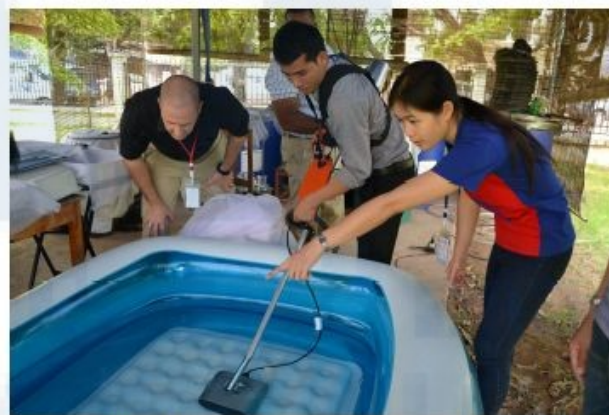
April 7, 2016. Dr. Ian Sutherland NMRC-A Testing Sonic Boom Apparatus for mosquito larval control
